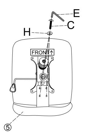
Note:Do not tighten screws fully until you have completed assembly.
